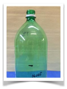
**MAKE A NOSE CONE**: Notice (on left photo) a felt tip marking which is located 6 inches from the top (of neck).
