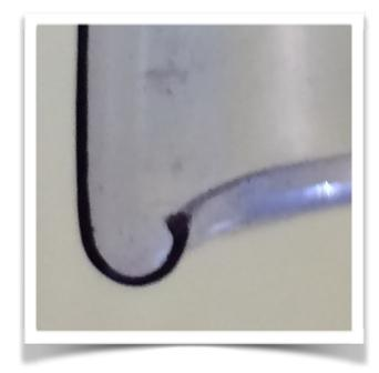
When temperature is right, push plastic cylinder down evenly, with equal flat pressure onto the hot plate. If the curl is forming on one side only, adjust the downward pressure to encourage the uncurled side to curl. When the curl is completely around circumference, IMMEDIATELY lift off hot plate and push over clay flower pot and hold in that position for about 15 seconds.
