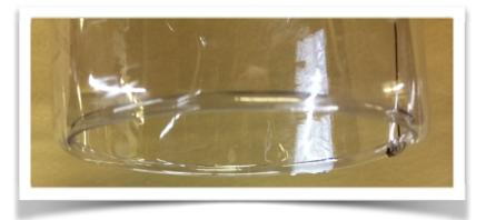
You will very lightly push the PETE cylinder to "feed" the plastic onto the hot saw blade. If one side is curling, while another side is not, it is because you need to push down equally so the curl
