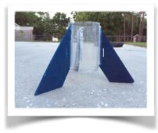
The construction of the Slideon Fin Assembly is more involved because a 3rd component is added to the Booster and Nose Cone. A cylinder is made from a soda bottle by removing the nose and bottom. One end of this cylinder is heated and formed into curl to make a structural re-enforcement ring.
