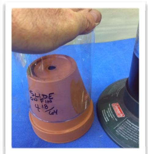
forms all the way around. When the completed inward plastic curl forms, you will pull immediately from the heat and then quench the soft molten ring over a upside-down clay flower pot. The tapered portion of the flower pot that comes in contact with the molten PETE plastic needs to be about 4” in diameter. This particular flower pot was about 4-1/2” at the top. When the molten PETE plastic comes in contact with the flower pot, it quenches it into a perfect plastic circle.
