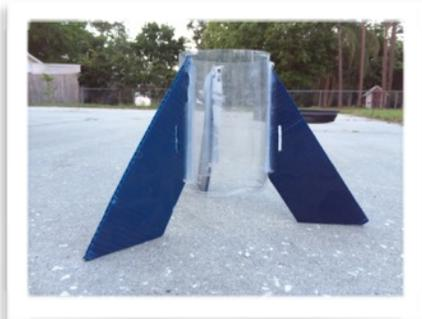
The construction of the Slide-on Fin Assembly is more involved because a 3rd component is added to the Booster and Nose Cone. A cylinder is made from a soda bottle by removing the nose and bottom. One end of this cylinder is heated and formed into curl to make a structural re-enforcement ring.
