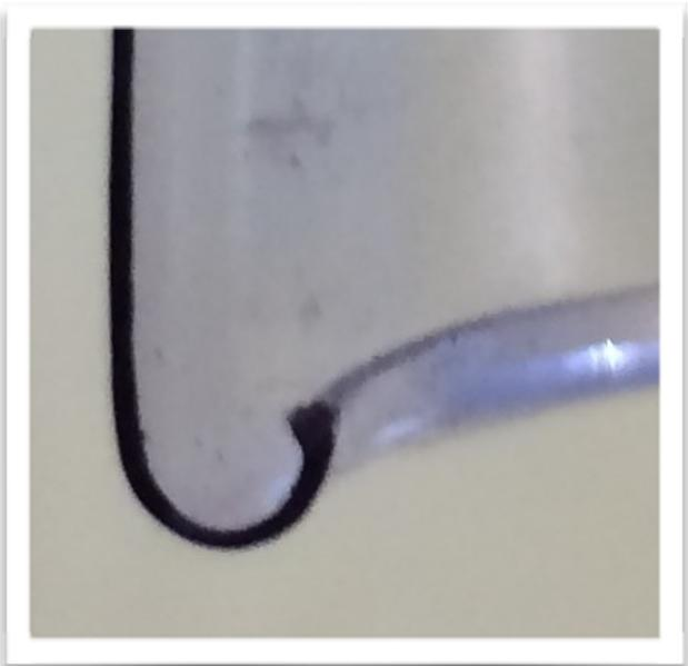
When temperature is right, push plastic cylinder down evenly, with equal flat pressure onto the hot plate. If the curl is forming on one side only, adjust the downward pressure to encourage the uncurled side to curl. When the curl is completely around circumference, IMMEDIATELY lift off hot plate and push over clay flower pot and hold in that position for about 15 seconds.
