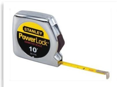
Hardware. [Flexible cloth/plastic dress maker tapes work well also]. The back side of the Stanley Diameter Scale measuring tape has a second scale for measuring diameters of round objects by wrapping the tape around the
